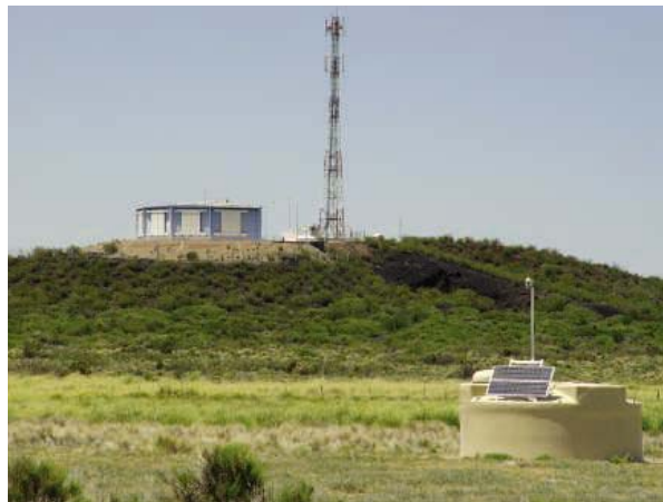
Cosmic dissonance. Auger’s particle detectors (foreground) and telescopes measure different energies for particles from space.
